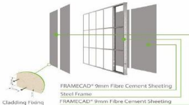
Fibre Cement sheeting and steel framing
